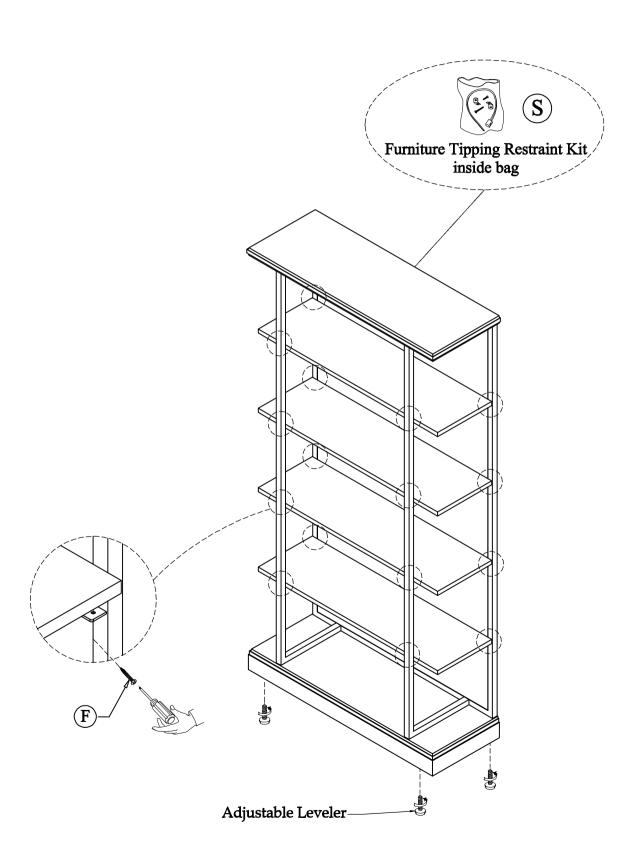
For product and personal safety, a Anti-Tip Restraint Kit has been included with this cabinet which can help to minimize the risk of the cabinet accidentally tipping forward,if used and properly installed
